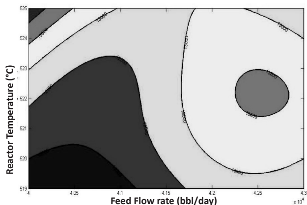
Figure 10: The effect of reactor temperature (°C) and feed flow rate (bbl/day) on formation of total cycle oil (bbl/day) (LCO and HCO).
