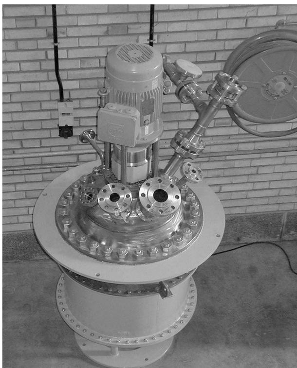
**Figure 3: 100 L pressure reactor (Disal Co., Iran) used for pilot scale preparation of Topanol A**
