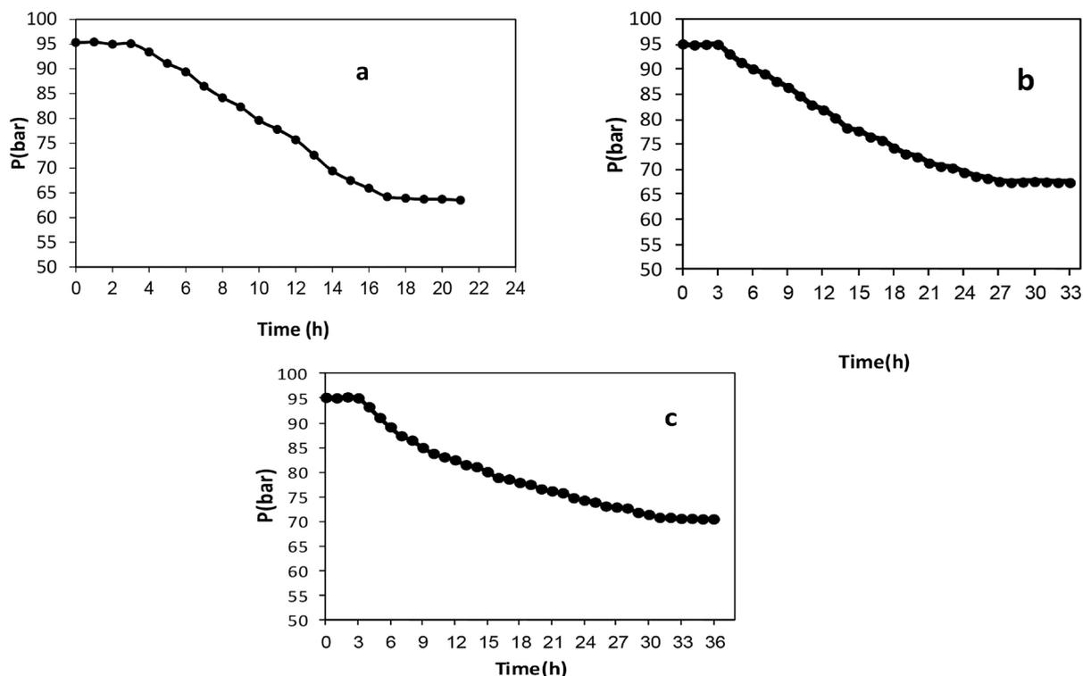
**Figure 4:** The change of pressure with time for natural gas hydrate formation: (a) in the presence of the kinetic inhibitor (0.5 wt.%) + EGME (0.5 wt.%), (b) in the presence of the kinetic inhibitor (0.5 wt.%) + EGMP (0.5 wt.%), (c) in the presence of the kinetic inhibitor (0.5 wt.%) + EGMB (0.5 wt.%).
