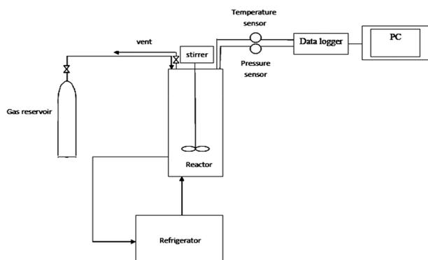
**Figure 1: Schematic representation of the experimental apparatus.**
