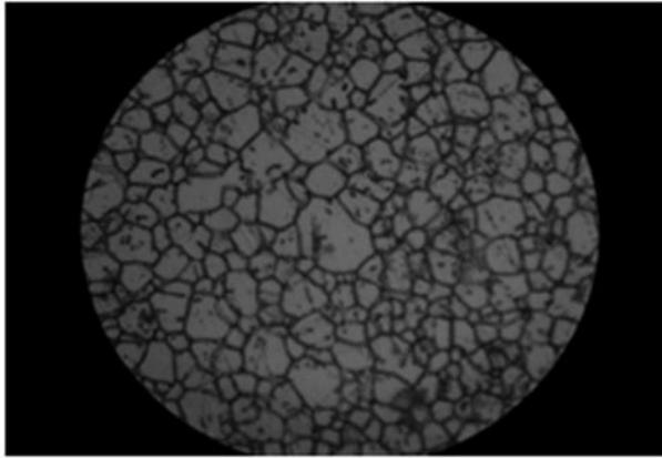
**Figure 2-** Optical microscope image of the sensitized sample of SS 304
