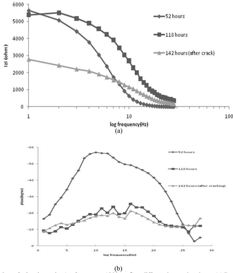
Figure 5- Bode plots of u-bend samples (surface area = 1200 mm<sup>2</sup>) at different immersion times; (a) Bode, (b) Bode phase
