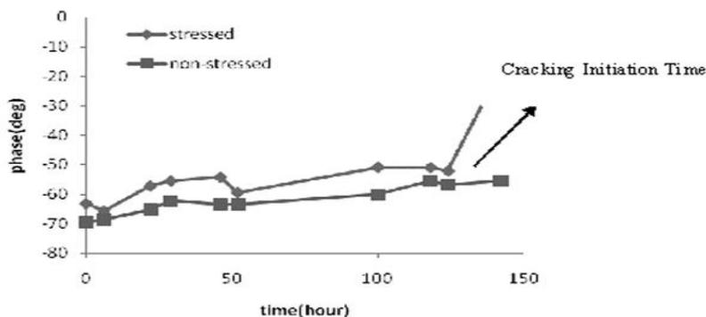
Figure 9- Phase-time plot of the stressed and non-stressed specimens at a frequency of 23.95 Hz
