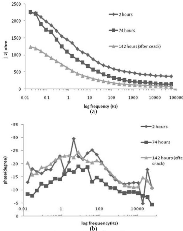
Figure 8- Bode plots of u-bend samples (surface area = 600 mm<sup>2</sup>) at different immersion times; (a) Bode, (b) Bode phase
