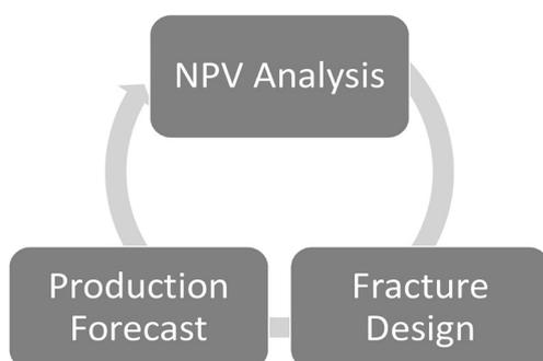
Different scenarios and treatment schedules have been designed to achieve distinctive features of different fracture lengths, then oil production is projected at different scenarios using the Eclipse
