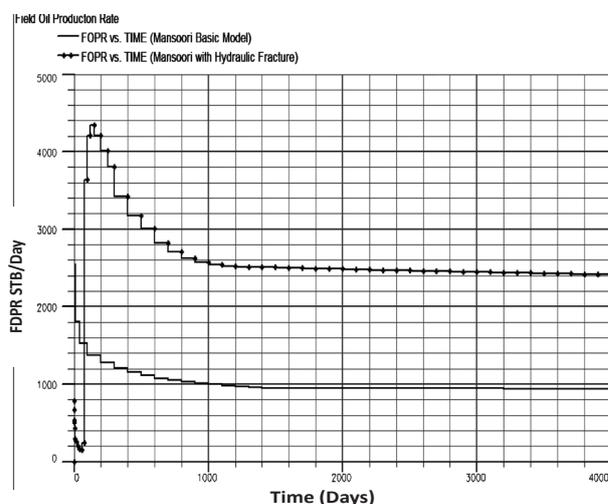
Figure 9: Oil production rate from a vertical well for MNS-Y before and after hydraulic fracturing simulation.
