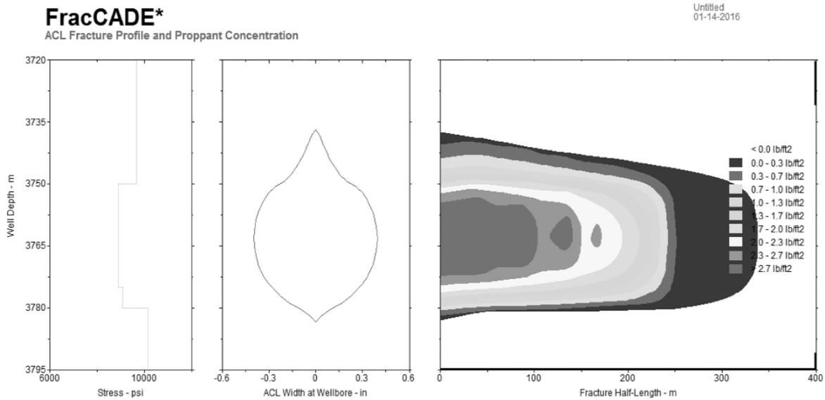
**Figure 4: Proppant concentration profile for well MNS-Y.**
