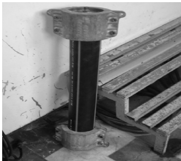
Figure 2: Pipe sample arrangements for burst test
