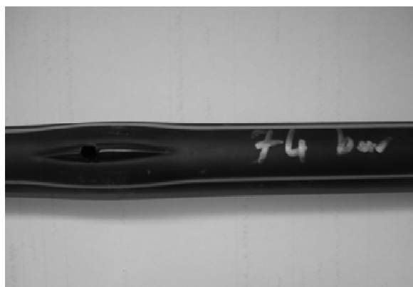
Figure 8: The pattern of ductile failure in polyethylene pipes
