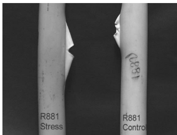
Figure 9: The pattern of pipe failures observed in burst tests for anti-rodent-added PE compounds
