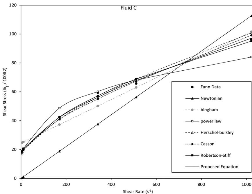
**Figure 9: Comparison of rheological models for fluid C.**
