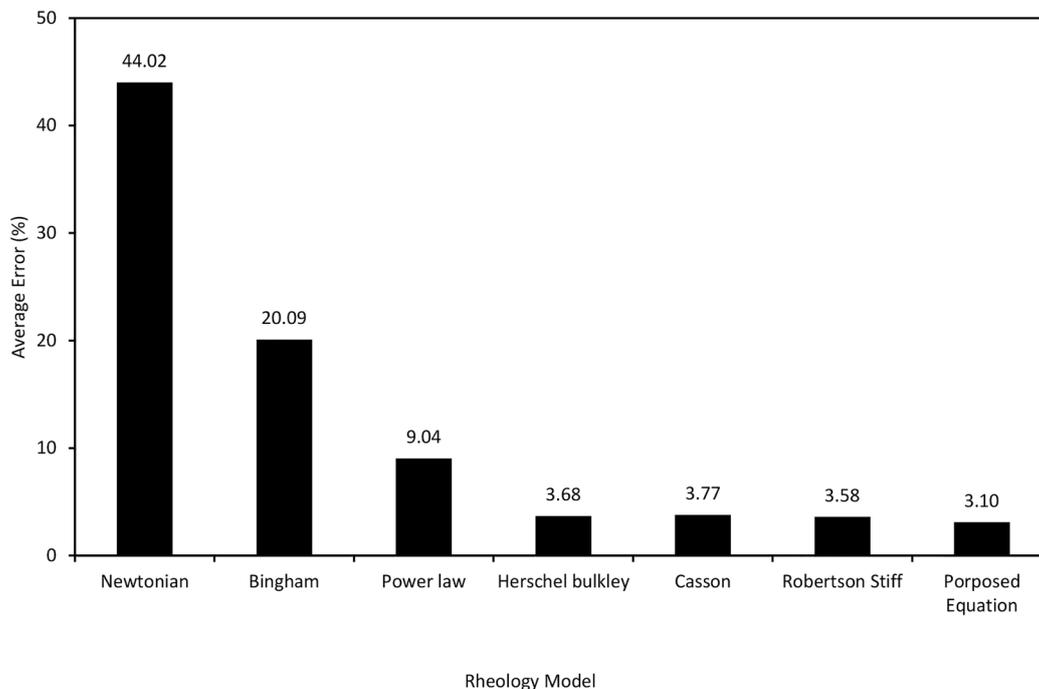
**Figure 13: Comparison between mean absolute average percent errors for all models.**
