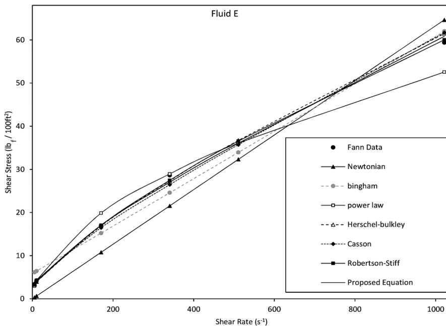
**Figure 11: Comparison of rheological models for fluid E.**
