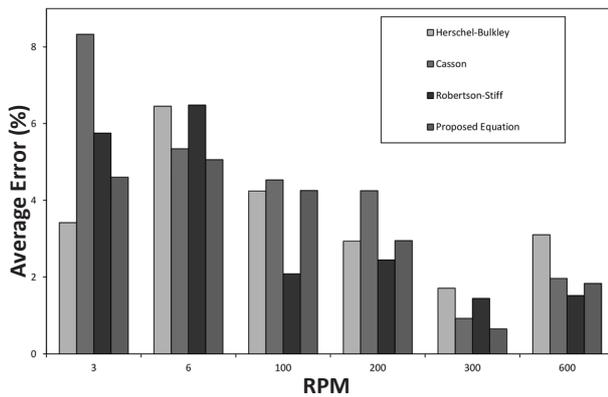
**Figure 14: absolute percent errors for Herschel-Bulkley, Casson, Robertson-stiff and proposed equation with different velocity.**
