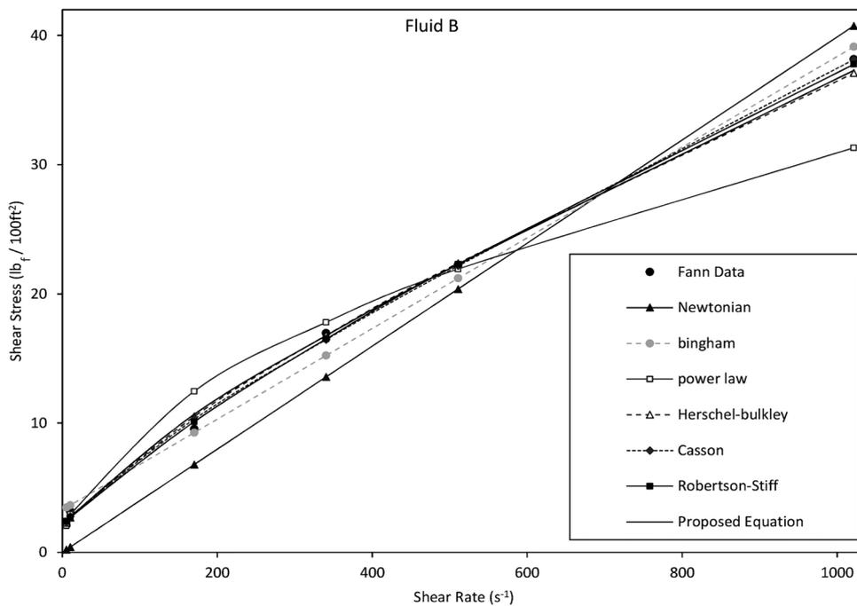
Figure 8: Comparison of rheological models for fluid B.
