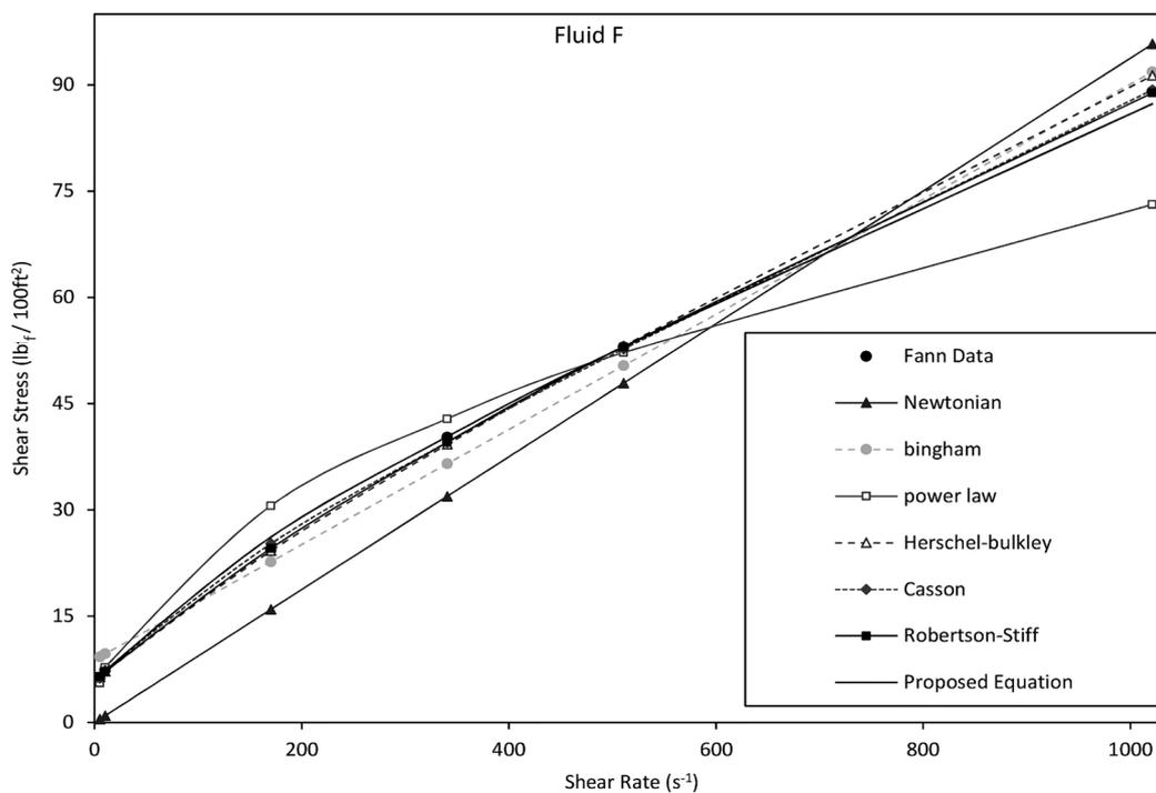
Figure 12: Comparison of rheological models for fluid F.
