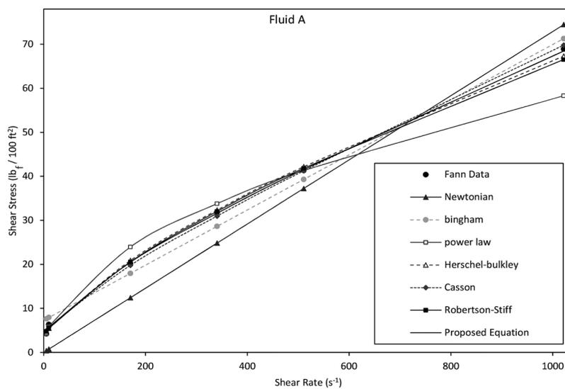
**Figure 7: Comparison of rheological models for fluid A.**
