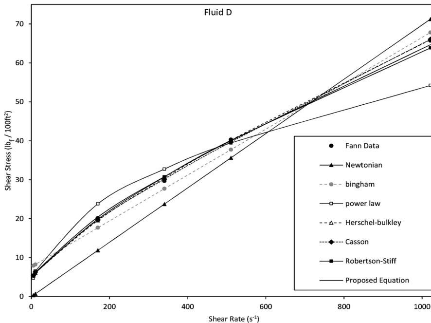
Figure 10: Comparison of rheological models for fluid D.
