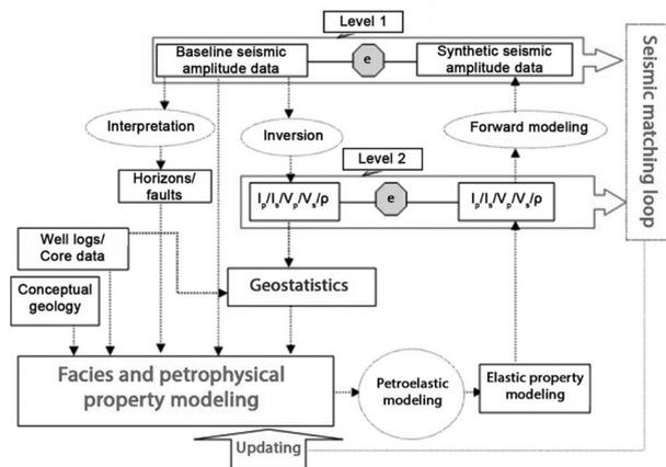
Figure 7: A typical workflow for seismic-constrained static reservoir modeling [1].
