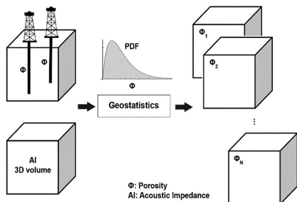
Figure 5: A schematic view of generating multiple equiprobable realizations of reservoir properties using geostatistical simulation [1].
