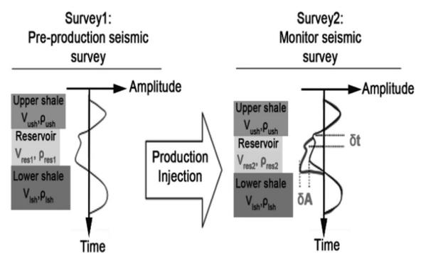
**Figure 9: The physical principle of time-lapse seismic reservoir monitoring; production or injection results in changes in P- and S-wave velocities and density, which appear as changes in amplitude and timing in the monitor seismic survey (adapted from [59]).**
