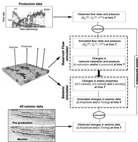
Figure 13: The Workflow of the quantitative integration of 4D seismic data in reservoir simulation process.
