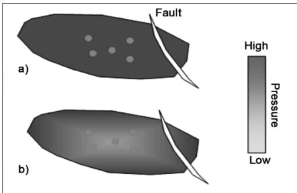
Figure 10: A schematic map of the reservoir pressure (a) before and (b) after production; green circles are the producer locations (adapted from [60]).
