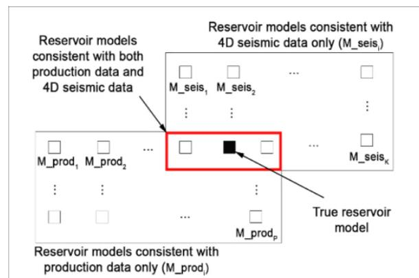
Figure 11: The basic philosophy of integrating 4D seismic data into the reservoir history matching process (adapted from [1]).
