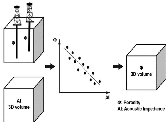
Figure 4: A schematic view of generating a static reservoir model based on deterministic relationships between seismic attributes and reservoir properties [1].
