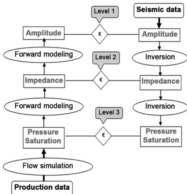
Figure 14: Joint seismic history matching can be performed at three different levels: amplitude, impedance, or pressure/saturation
