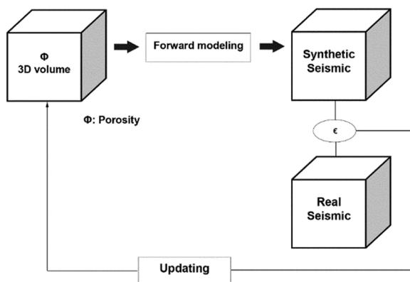
**Figure 6: A schematic view of reservoir model building and updating by the seismic matching loop process [1].**
