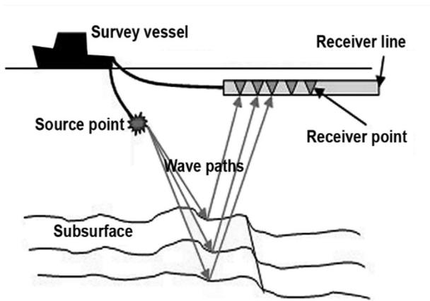
Figure 2: Seismic reflection data are typically acquired by transmitting energy into the Earth and recording the reflected energy from subsurface geological boundaries.
