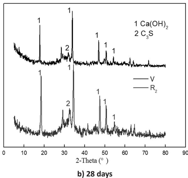
Figure 3: XRD pattern of specimen V and the specimen  $\text{R}_2$ .
