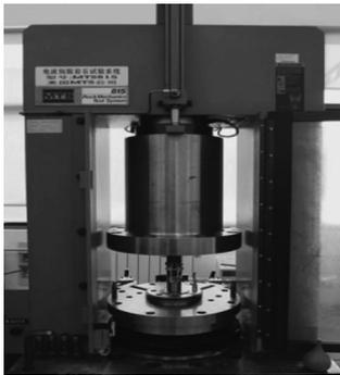
Figure 5: The experimental set-up of the creep test of rock.
