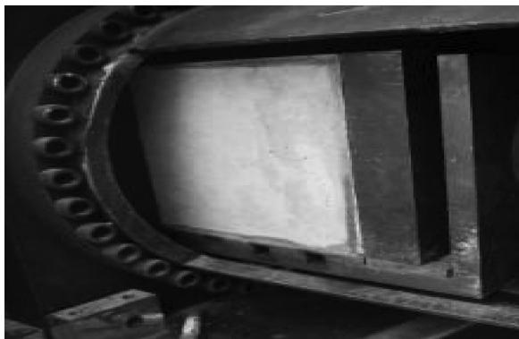
Figure 4: Experiment core for fracturing (300mm×300mm×300mm).
