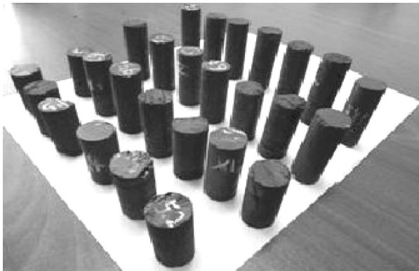
Figure 3: The coal sample of compression test (Φ25).
