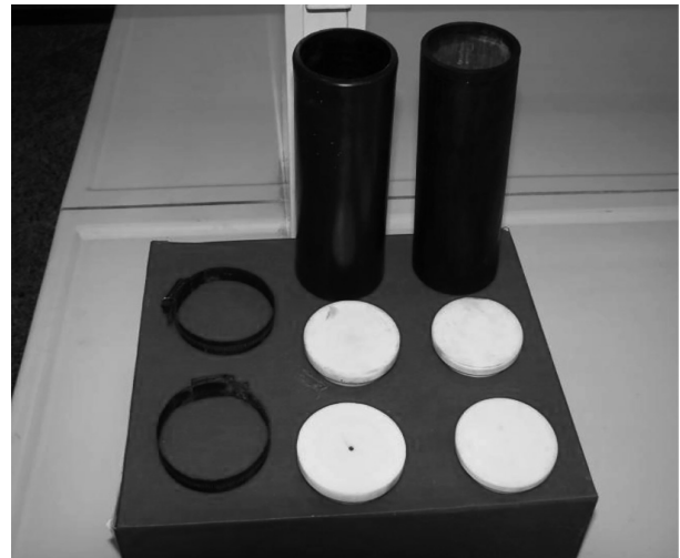
Figure 2: Cylindrical rubber mold ready for placement in a pressure curing chamber.
