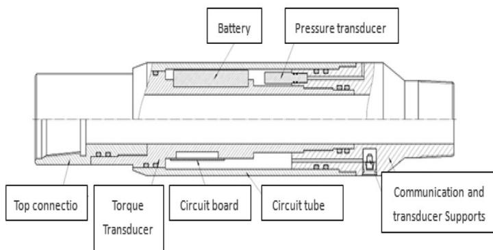
Figure 7: Tester structure diagram.
