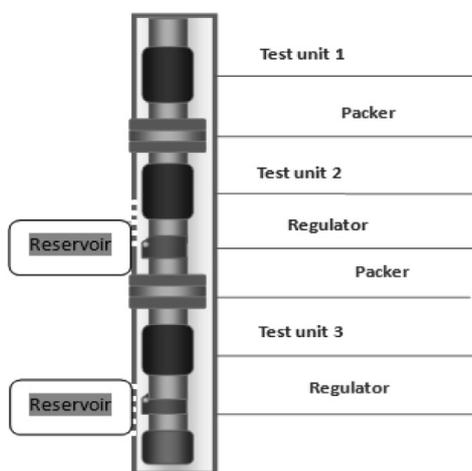
Figure 8: A schematic diagram of test process.
