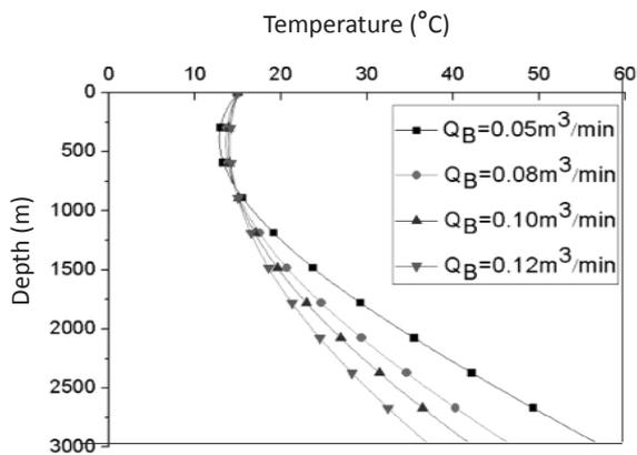
Figure 4: Wellbore temperature profiles and water injection rate curves.
