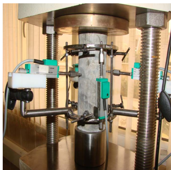
Figure 3: Uniaxial compressive strength tester equipped with axial and radial strain gauges.
