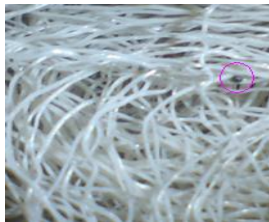
Figure 4: The stained product due to the degraded organomodified clay is shown inside the circle.
