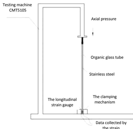
Figure 3: The buckling experimental device of slender string.
