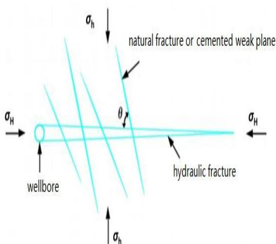
Figure 3: A schematic plot of joint network system.
