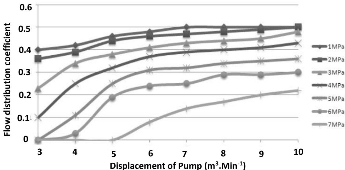
Figure 5: Relationship between different reservoir stresses and the influence of the flow within the cluster of the Chang 8 reservoir in Jihe oil field.
