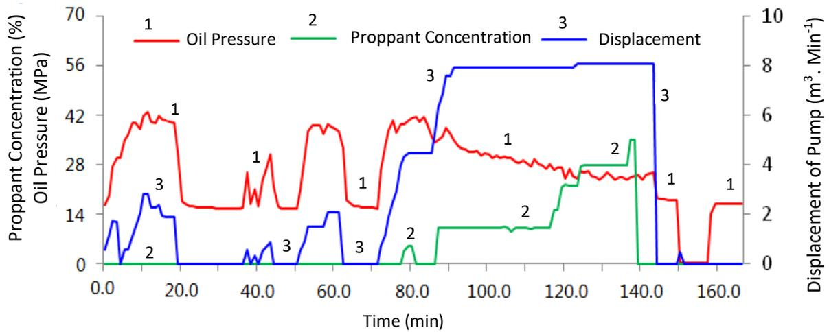
Figure 4: Segmented clusters fracturing construction graph of 8 sections.
