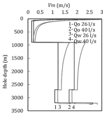
Figure 8: Relationship between annulus velocity and displacement.
