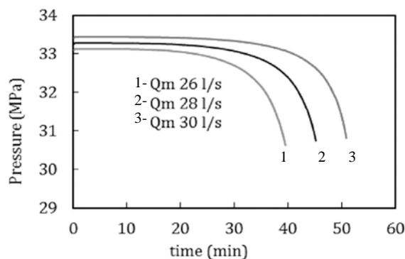
**Figure 11: Bottom-hole pressure versus time during gas kick.**
