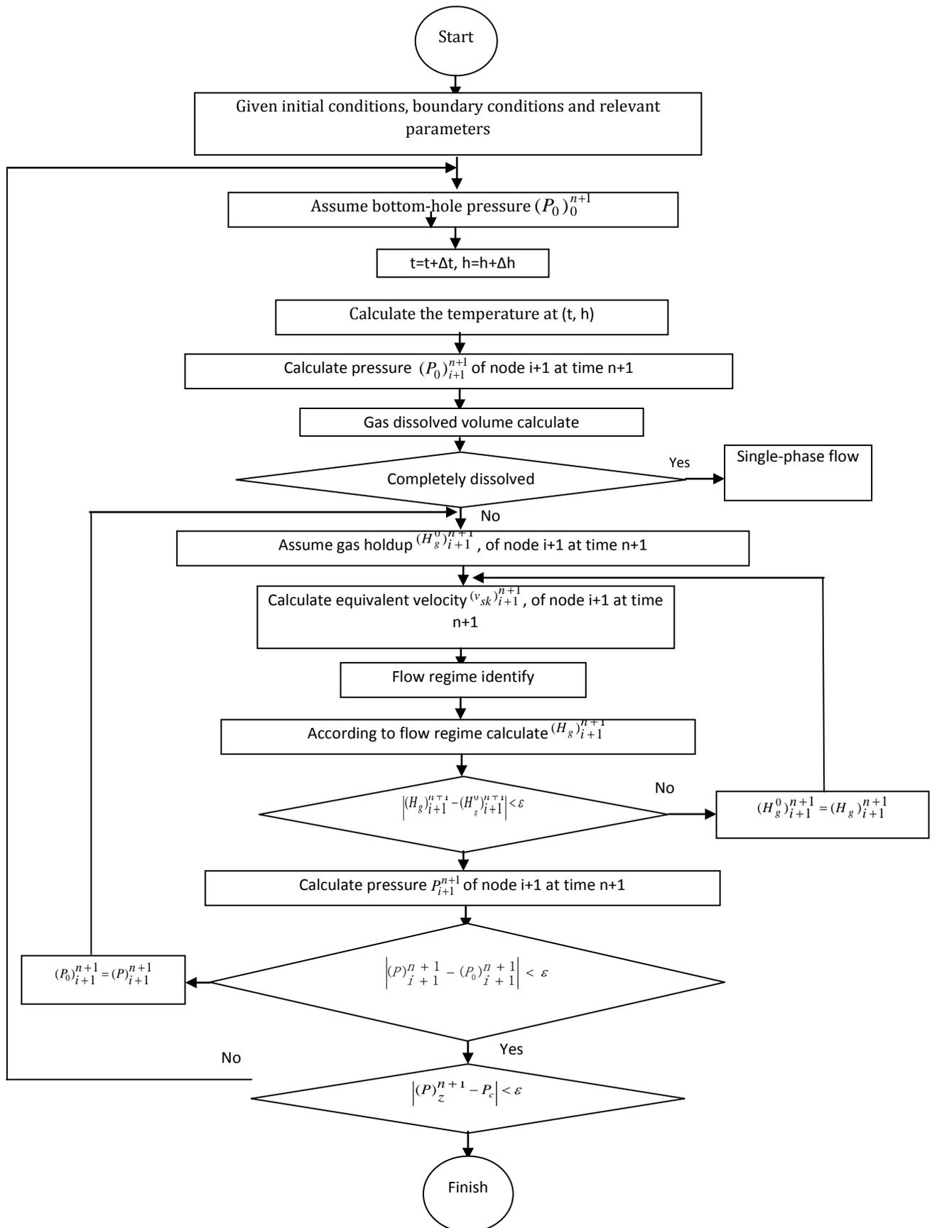
Figure 2: The calculation model of gas kick.
