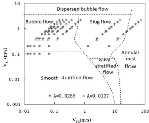
Figure 1: Possible flow type in an annulus.
