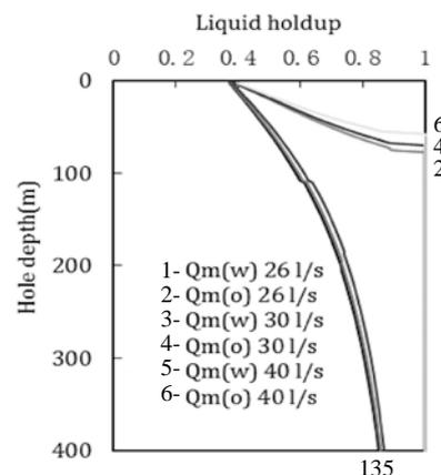
Figure 6: Relationship between liquid holdup and displacement.
