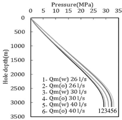
Figure 7: Relationship between annulus pressure and displacement.
