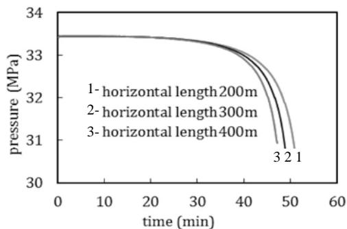
**Figure 10: Bottom-hole pressure versus time during gas kick.**
