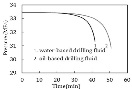
Figure 9: Bottom-hole pressure versus time during gas kick.
