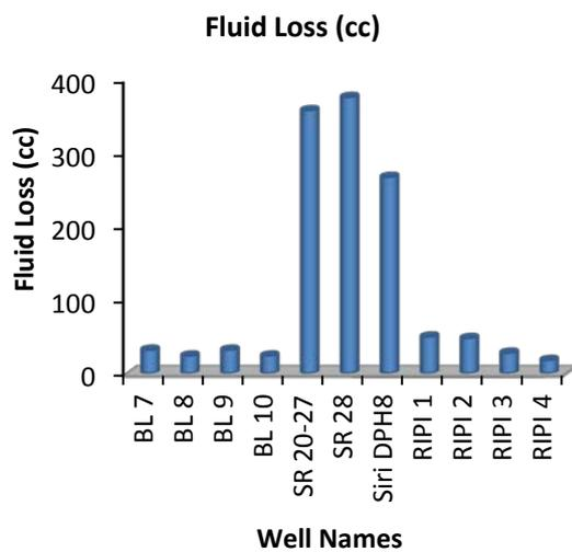
Figure 11: Fluid loss value of all the cement slurry systems
