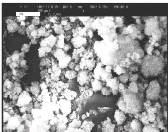
Figure 4: The SEM image of HSL particles with 750X magnification
