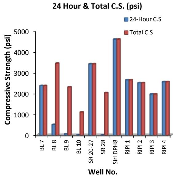
Figure 12: Compressive strength development for all the cement systems
