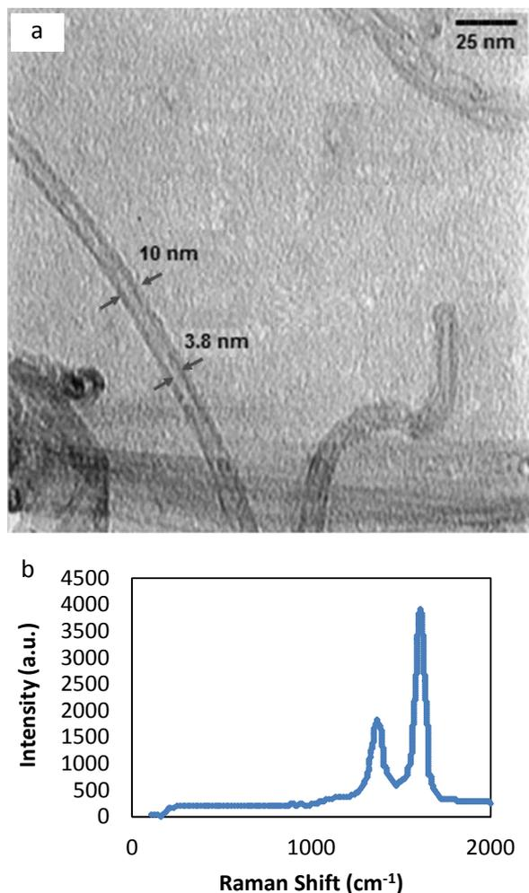
**Figure 1: a) TEM image and b) Raman spectrum of the synthesized MWNT**
