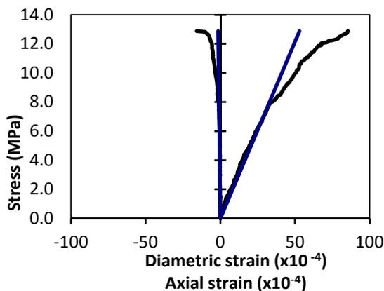
Figure 7: Axial and radial stress strain curve for slurry sample number 1
