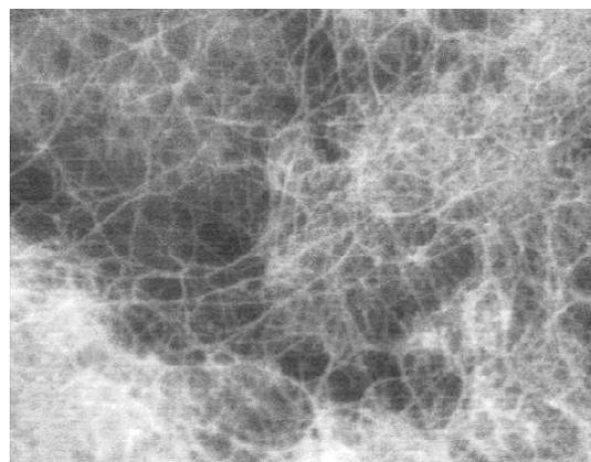
Figure 6: SEM photograph of the best SWNT's sample
