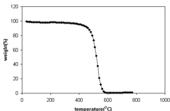
Figure 5: TGA analysis graph for the best SWNT's sample
