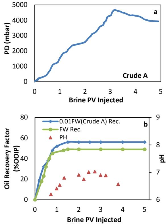
Figure 6: Oil recovery, pressure drop, and pH evolution during secondary recovery experiment on A5
