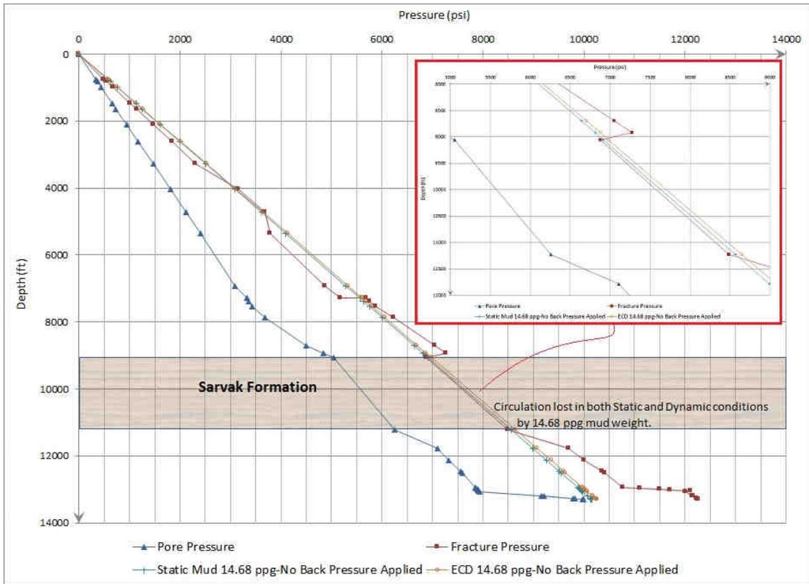
Figure 2: Operation window, static and dynamic BHP using a MW of 14.68 ppg at a pump rate of 767 gpm
