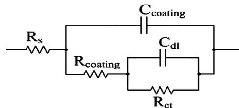
Figure 2: Equivalent electrical model of the coated mild steel
