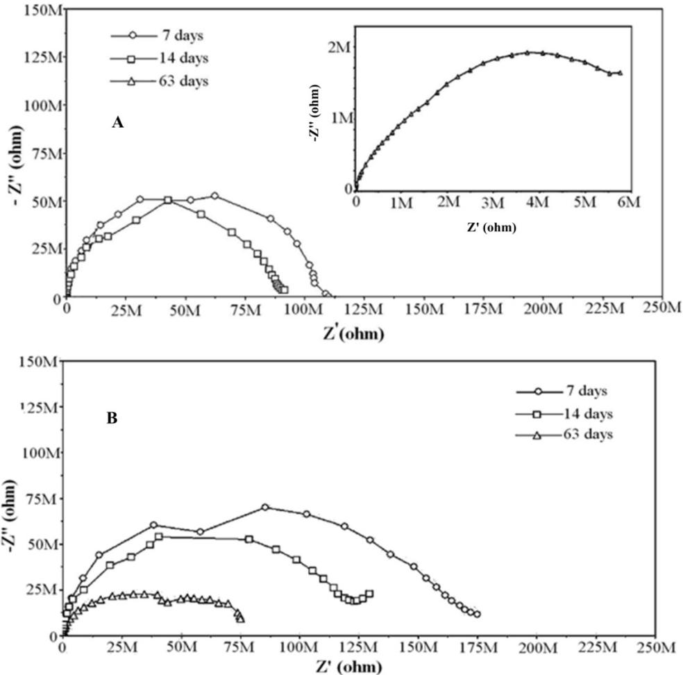
Figure 1: Typical Nyquist diagrams of ZP<sub>b</sub> (A) and ZAP<sub>b</sub> (B) during different immersion times in a 3.5 wt.% NaCl solution
