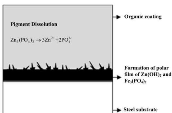
**Figure 3: Precipitation of the phosphate pigment and the increment of surface polarity**
