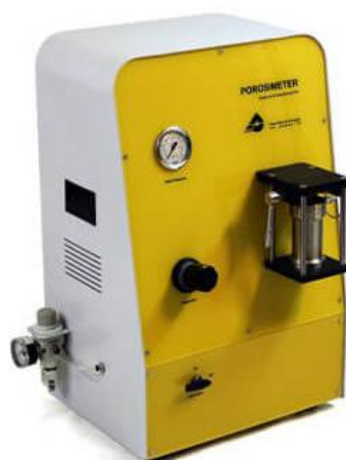
Fig. 3 A schematic of helium porosimeter device.
