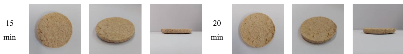
Fig 13. Images of Core 17 at different time intervals after exposure to 15 wt.% hydrochloric acid and 3 wt.% acetic acid solution with seawater.
