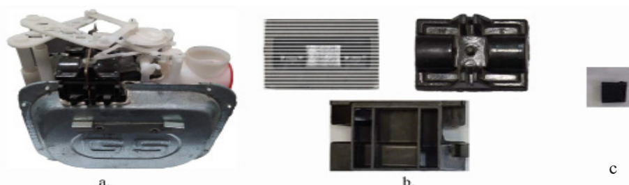
Fig. 1. a A conventional diaphragm gas meter with Bakelite valves, b. the two parts of Bakelite valves (moving lid and the seat) used in the present research, c. the prepared sample for XRD, AFM and SEM.
