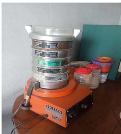
Figure 3L: A digital sieve shaker. sieve.
