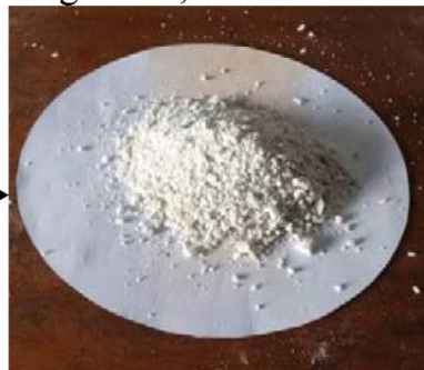
Figure 3d, Site 2: Grinded baryte
