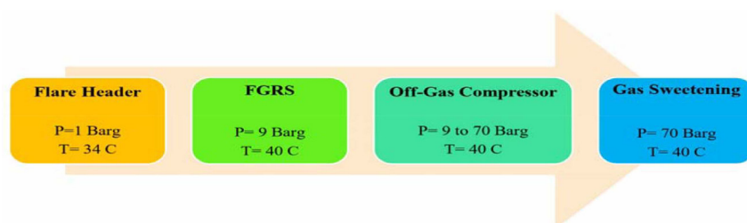
Fig. 3 The Second Scenario Block Flow Diagram.
