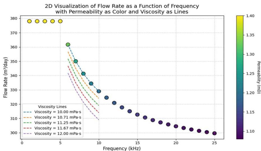
**Fig. 3** Visualization of oil production rate as a function of acoustic wave frequency, core permeability, and oil viscosity, emphasizing key reservoir characteristics and optimal wave stimulation conditions.
