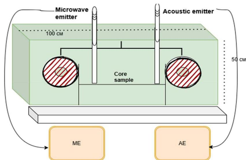
Fig. 1. Schematic of the experimental setup for combined acoustic and HF wave exposure.
