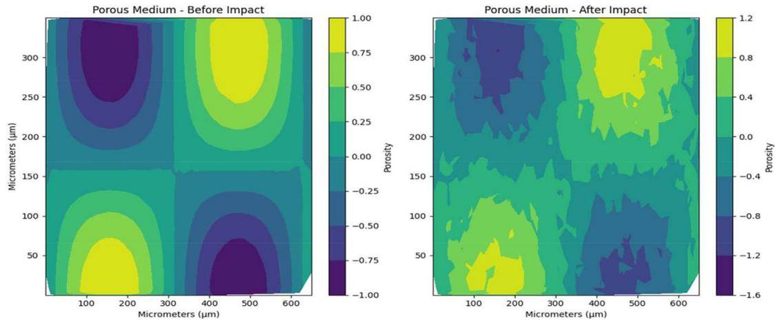
Fig. 4 Porosity Distribution in a Porous Medium Before and After Elastic Wave Stimulation.
