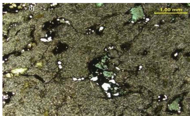
b. JIN201, 4168.55 m, andesitic volcanic breccia, microfractures, chlorite, zeolite, and silicon; asphalt observed in microfractures
