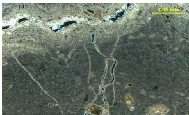
a. JIN204, 4287.29 m, welded tuff, elongated siliceous semi-filled vesicles locally; asphalt observed in pores and microfractures.
