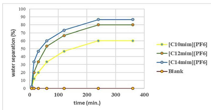
**Fig. 2** Effect of molecular weight on demulsification efficiency of  $[C_{10-14}\text{mim}][\text{PF}_6]$  ILs
