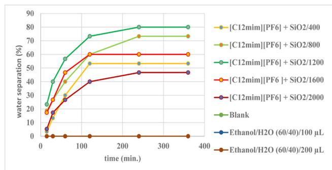
**Fig. 4** Water separation by nanosilica coated with [C<sub>12</sub>mim][PF<sub>6</sub>] ionic liquid in ethanol/water.
