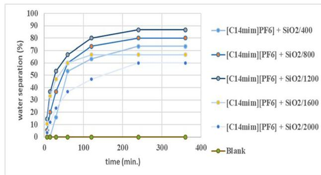
**Fig. 5** Water separation by nanosilica coated with [C<sub>14</sub>mim][PF<sub>6</sub>] ionic liquid in ethanol/water (60/40) solvent mixture.
