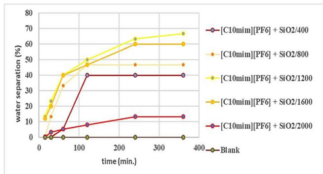
**Fig. 3** Water separation by nanosilica coated with [C<sub>10</sub>mim][PF<sub>6</sub>] ionic liquid in ethanol/water (60/40) solvent mixture.
