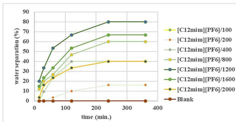
**Fig. 1** Water separation (%) by different concentrations of  $[C_{12}\text{mim}][PF_6]$  ionic liquid.
