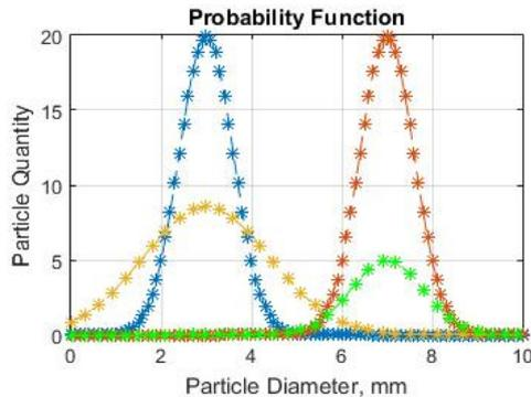
Fig. 1 Particle Diameter Dispersion Functions.
