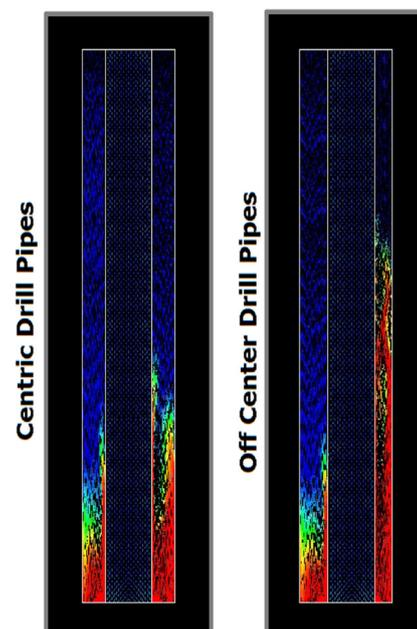
Fig. 8 Particle Movement when Drill Pipes are at Hole Center or off Center
