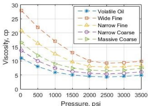
Figure 5. Viscosities for Particle in Oil Mixtures.
