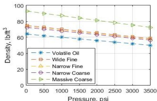
Fig. 4 Densities for Particles in Oil Mixtures.
