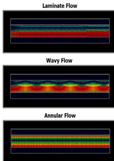
Fig. 6 Flow Patterns in Horizontal Pipe Model.
