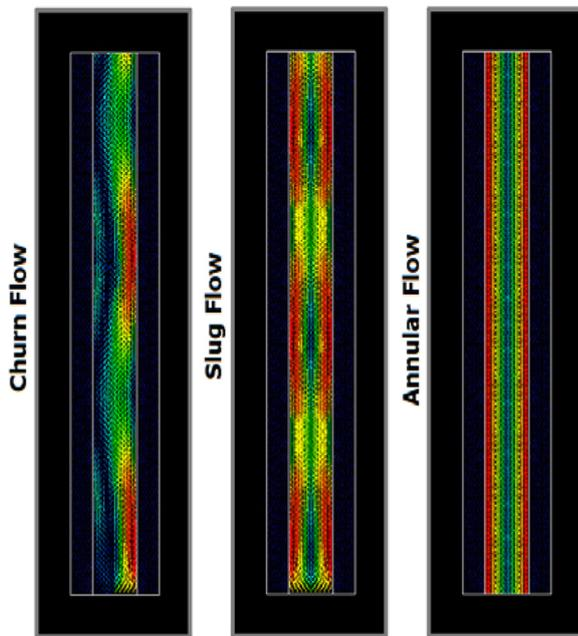
Fig. 7 Flow patterns in vertical tubing model.
