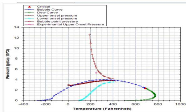
**Fig. 3** Asphaltene precipitation phase envelope for the reservoir sample (250 °F).
