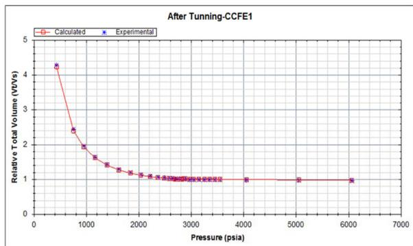
**Fig.1** Matching the CCE test results for the fluid sample.
