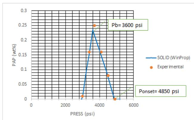
**Fig. 2** Asphaltene precipitation curve generated using WinProp.
