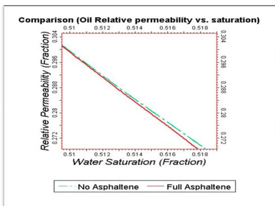
**Fig. 11** Comparing relative oil permeability for two simulation cases: No Asphaltene and Asphaltic in Eclipse (indicating a slight wettability alteration due to asphaltene deposition).
