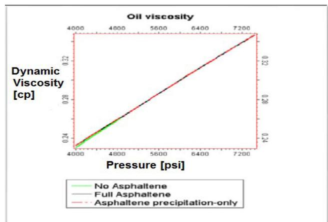
Fig. 9. Comparing viscosity in three simulation cases: No asphaltene, precipitation-only, and Full-asphaltene in Eclipse (showing viscosity alteration due to asphaltene precipitation).
