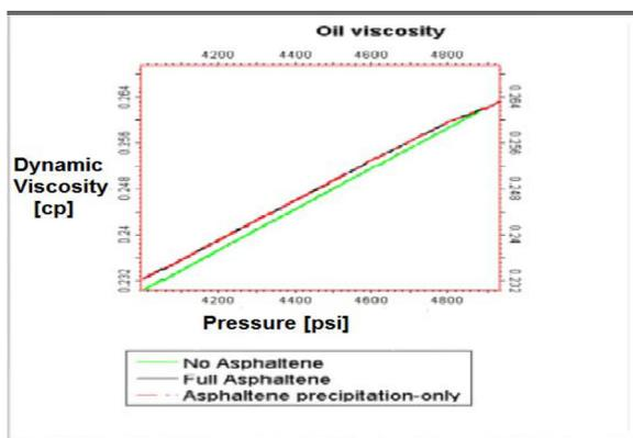
**Fig. 10** A closer view of the difference in viscosity of three simulation cases: No asphaltene, precipitation-only, and Full Asphaltene in Eclipse.
