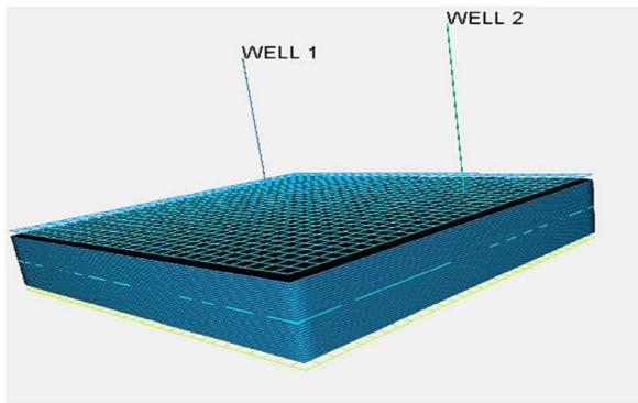
Fig. 4 3D reservoir discretization in Cartesian system.
