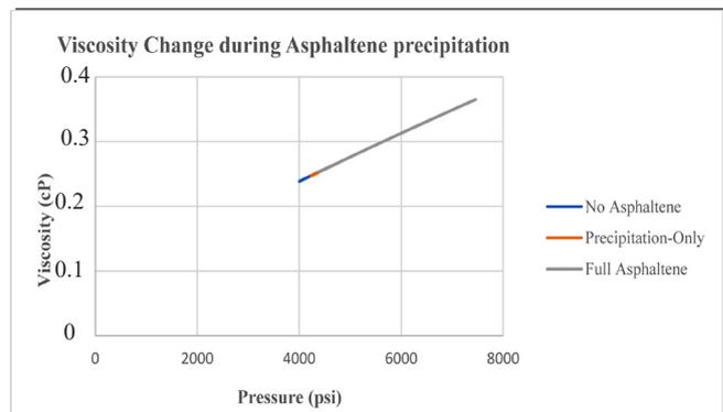
Fig. 8 Comparison of viscosity in three simulation cases: No asphaltene, precipitation-only, and Full-asphaltene precipitation/ deposition in GEM.
