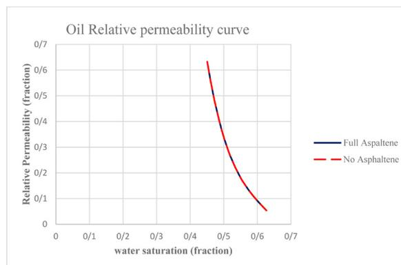
**Fig. 12** Comparing relative oil permeability for two simulation cases: No Asphaltene and Asphaltic in GEM (indicating unchanged wettability due to asphaltene deposition).
