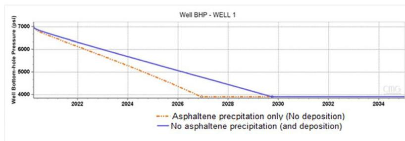
Fig. 5 Comparison of declining bottom-hole pressure in two simulation cases: no asphaltene and asphaltene precipitation-only in GEM.
