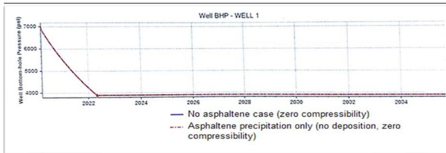
Fig. 6 Matching bottom-hole pressure in two models with zero compressibility in GEM.
