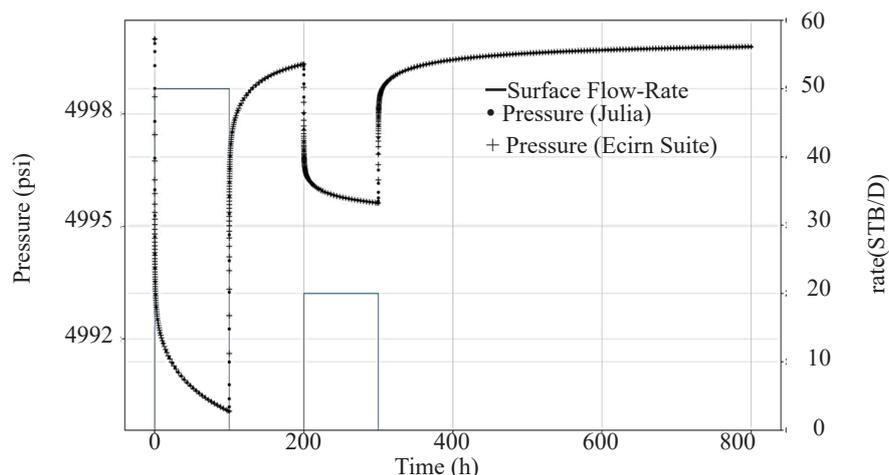
Fig. 4 Overlay of Simulated pressures from Industry Software and Julia.
