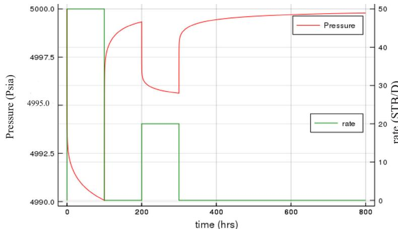
Fig. 3 Simulated pressure response using Industry software.
