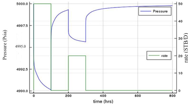
Fig. 2 Simulated pressure response using Julia.
