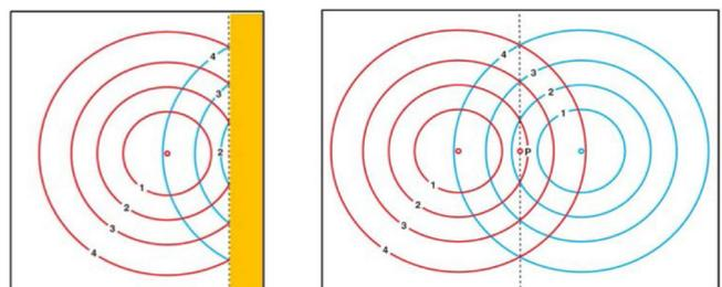
**Fig. 1** Single sealing fault with corresponding image well (after kappa).
