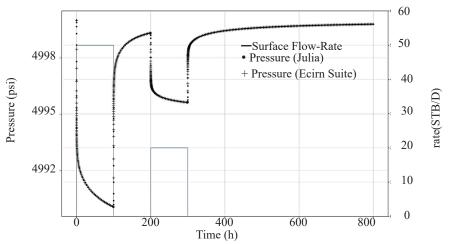
Fig. 4 Overlay of Simulated pressures from Industry Software and Julia.
