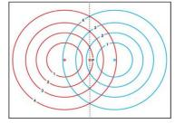
Fig. 1 Single sealing fault with corresponding image well (after kappa).
