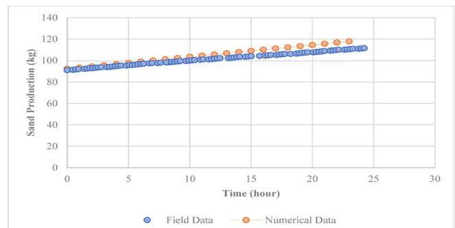
Fig. 7 Comparison of field data and simulation data for the amount of sand produced in the third interval.
