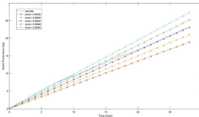
Fig. 4 Select the best sand production coefficient.
