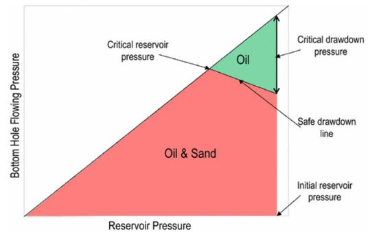
Fig. 1 An example of critical drawdown pressure chart [13].
