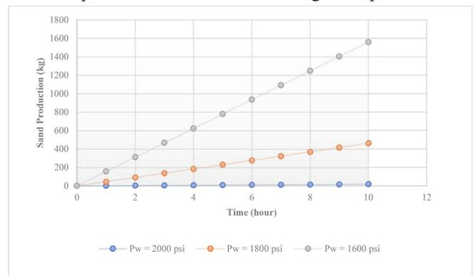
**Fig. 10** Sensitivity analysis on accumulated sand production based on wellbore pressure parameter.
