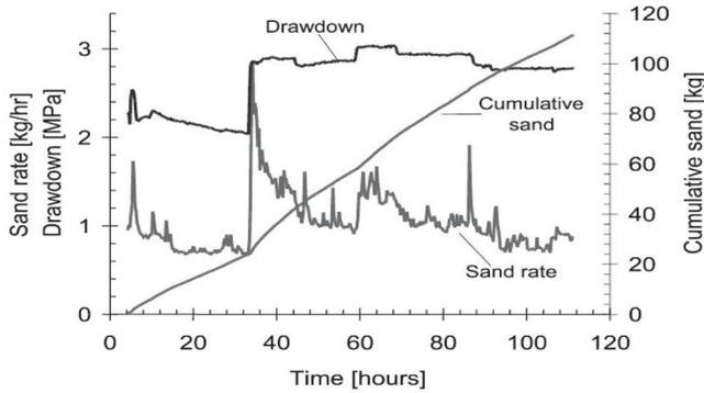
Fig. 3 Sand rate, cumulative sand production, and drawdown pressure for mentioned well during 120 hours period [20].
