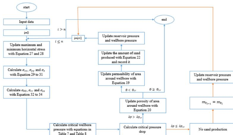
Fig. 2 The process of calculating the amount of sand production.
