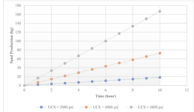
**Fig. 9** Sensitivity analysis on accumulated sand production based on uniaxial compressive strength parameter.
