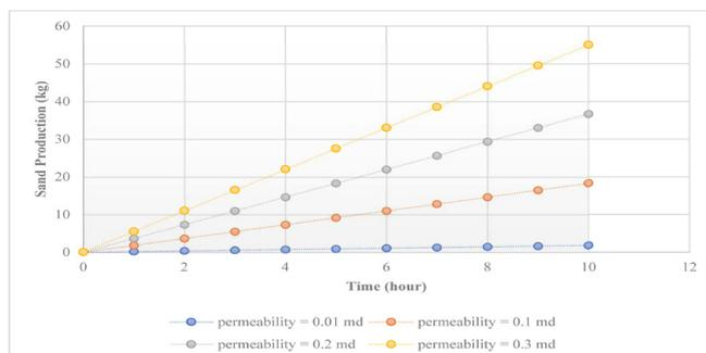
**Fig. 8** Sensitivity analysis on accumulated sand production based on permeability parameter.
