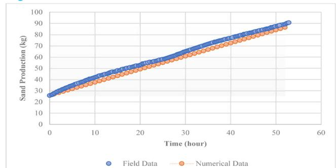
Fig. 6 Comparison of field data and simulation data for the amount of sand produced in the second interval.
