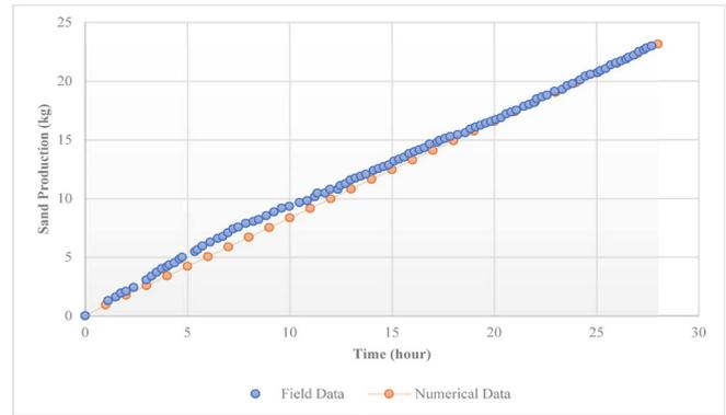
Fig. 5 Comparison of field data and simulation data for the amount of sand produced in the first interval.
