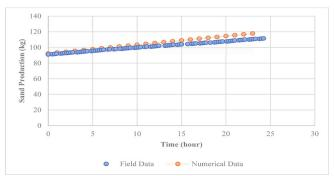
Fig. 7 Comparison of field data and simulation data for the amount of sand produced in the third interval.
