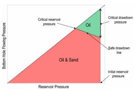
Fig. 1 An example of critical drawdown pressure chart [13].
