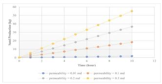
Fig. 8 Sensitivity analysis on accumulated sand production based on permeability parameter.
