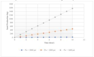
**Fig. 10** Sensitivity analysis on accumulated sand production based on wellbore pressure parameter.
