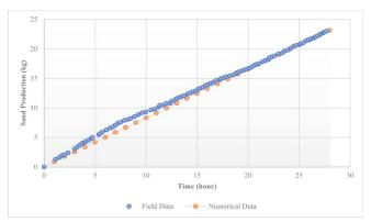
Fig. 5 Comparison of field data and simulation data for the amount of sand produced in the first interval.
