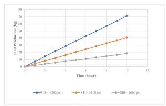
Fig. 11 Sensitivity analysis on accumulated sand production based on maximum horizontal stress parameter.
