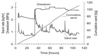
**Fig. 3** Sand rate, cumulative sand production, and drawdown pressure for mentioned well during 120 hours period [20].
