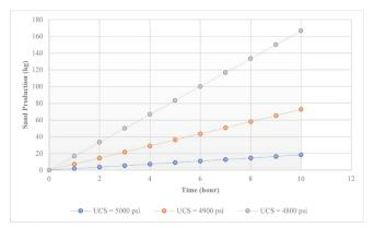
Fig. 9 Sensitivity analysis on accumulated sand production based on uniaxial compressive strength parameter.
