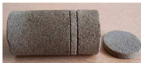
Fig. 1 Interception position of frozen core after laboratory displacement experiment.
