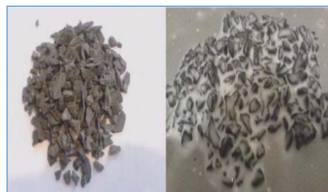
Fig 6 Shale Recovery test (left: before the test, Right: after tests).
