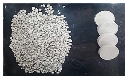
Fig 3 Shale samples converted to shale wafers.
