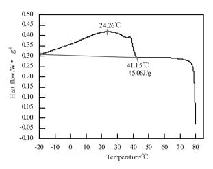
Figure 2a: Wax content of the oil sample before the treatment.
