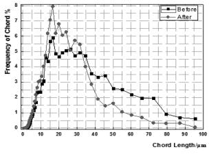
Figure 4: The chord length distribution (CLD) of the oil sample.
