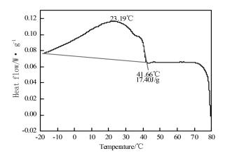
Figure 2b: Wax content of the oil sample after the treatment.
