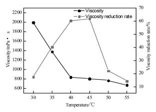
Figure 5: Effect of compound bacteria on viscosity of crude oil.
