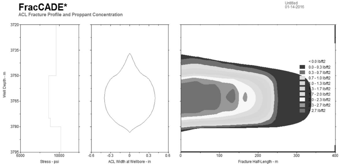
**Figure 4: Proppant concentration profile for well MNS-Y.**
