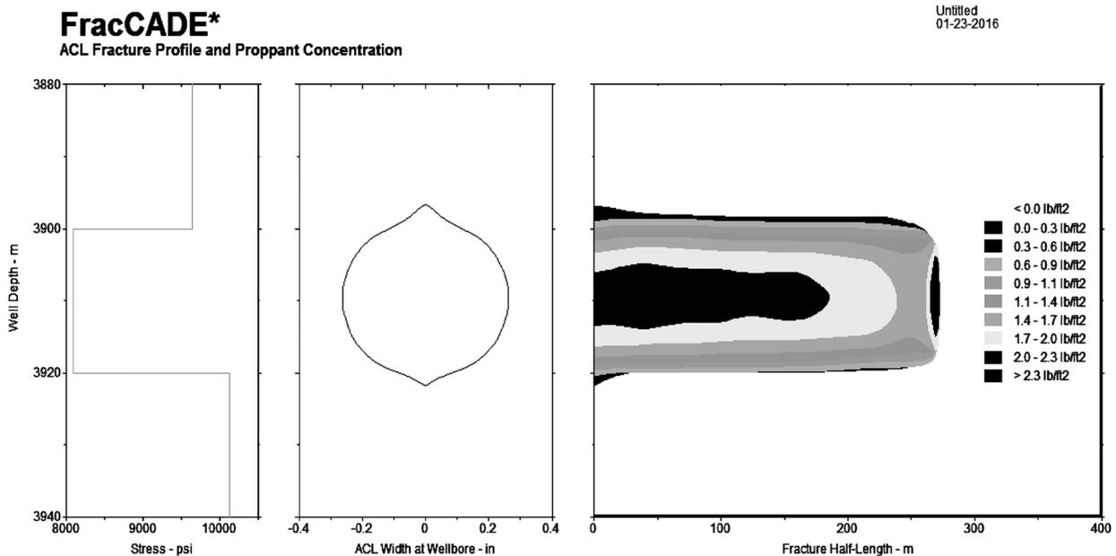
**Figure 5: Proppant concentration profile for well AZ-X.**
