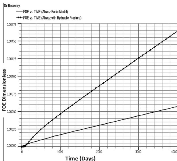
Figure 6: Oil recovery factor for Ahwaz reservoir before and after hydraulic fracturing simulation.
