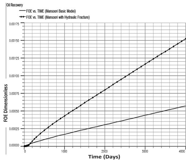
Figure 7: Oil Recovery factor for mansori reservoir before and after hydraulic fracturing simulation.
