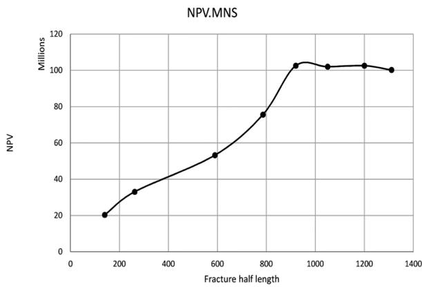
Figure 2: NPV versus fracture length for well MNS-Y.
