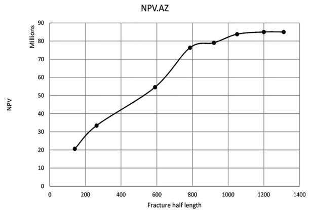
Figure 3: NPV versus fracture length for well AZ-X.
