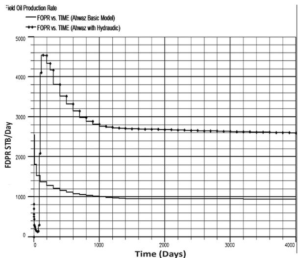
Figure 8: Oil production rate from a vertical well for AZ-X before and after hydraulic fracturing simulation.
