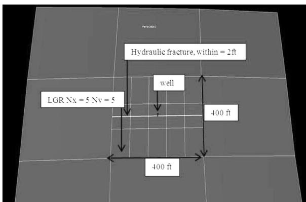
Figure 1: Fracture and wellbore LGR used in the model.
