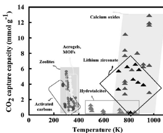
Figure 2: CO<sub>2</sub> capturing properties versus sorption temperature for various solid porous sorbents.
