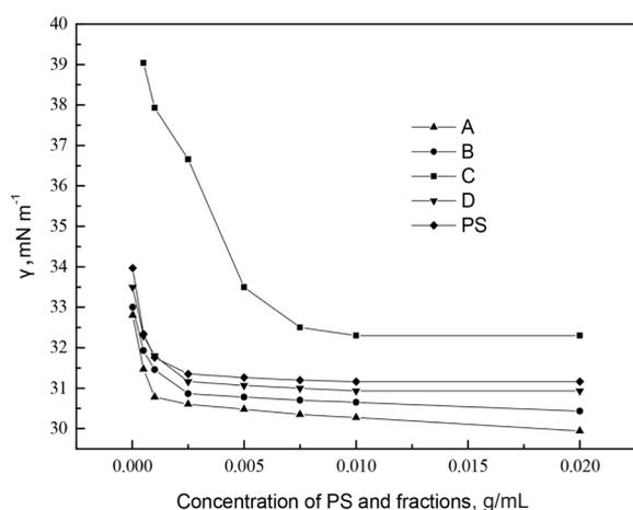
Figure 1: Surface-tension curves of PS and its fractions.
