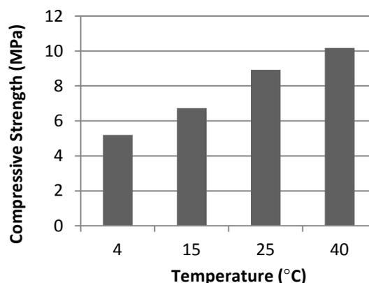
Figure 2: Effect of temperature on compressive strength [1].
