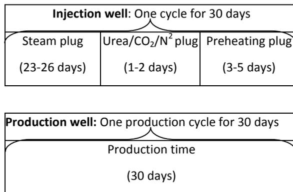
Figure 9: A scheme of a single-cycle injection
