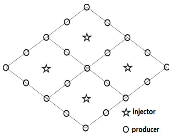
Figure 3: A schematic of 4 inverted nine-spot well patterns
