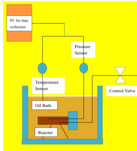
**Figure 2: A schematic of urea decomposition reactor**
