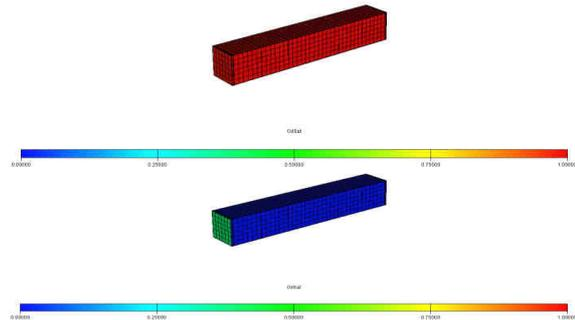
Figure 3: 6-stacked matrix block model showing the 3D saturation in the initial state (a) and after 20 years of production (b)
