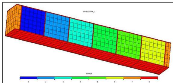
Figure 2: 6-stacked matrix block model showing the numerical grid block division with an x-z cross section at y=6 (dummy blocks, orange; fractures system, red; matrix blocks, remaining colors)
