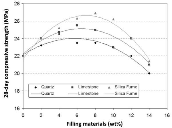
Figure 5: 28-day compressive strength of the cement blends
