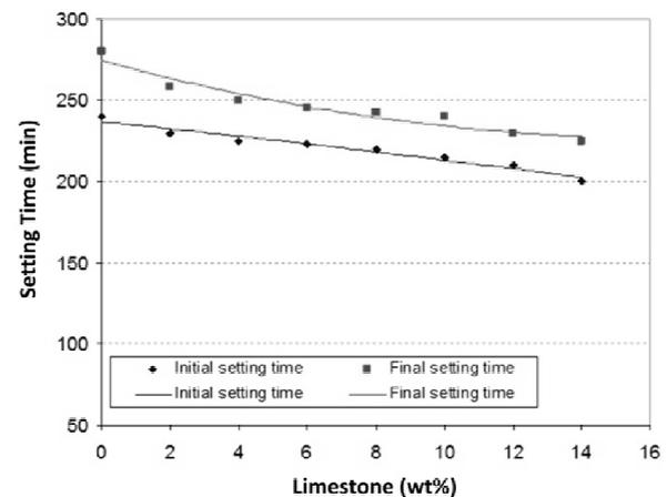
Figure 3: Effect of limestone powder on the initial and final setting times of cement
