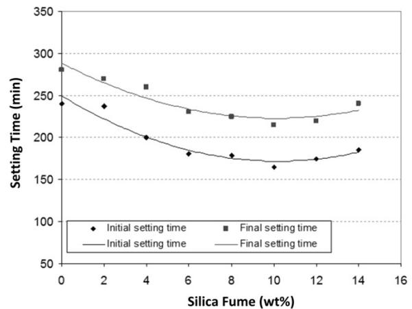
Figure 2: Effect of silica fume on the initial and final setting times of cement
