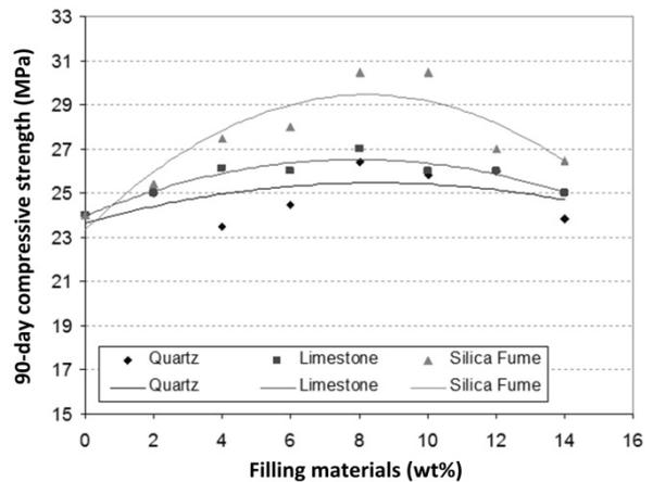
Figure 6: 90-day compressive strength of the cement blends
