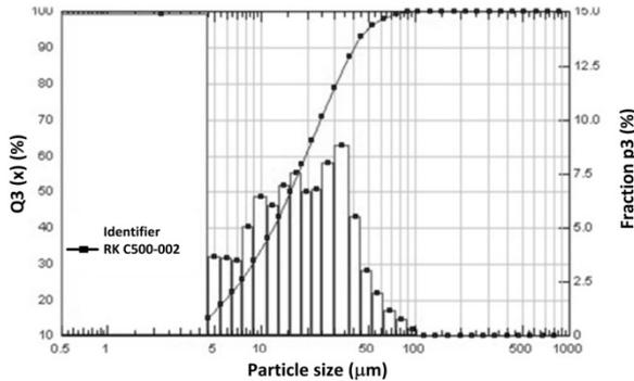
Figure 1: PSD-curve of class G oil well cement
